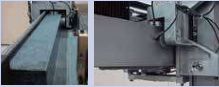
Integrated Y-Axis in Granite Table
