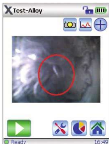
Example of 10 mm spot collimation
