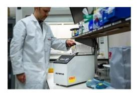
The BTX III X-ray diffraction (XRD) analyzer from Olympus Scientific Solutions offers fast, dependable quantitative mineralogy of both major and minor components in a small, benchtop design.
