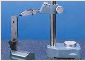
Setting a dial test indicator to a long-gauge-block stack attached to the base with a D-type connector
