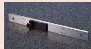
Coupling holes in long gauge blocks
