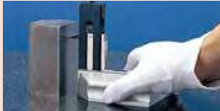
Marking a workpiece using the base, a holder and the scriber point
