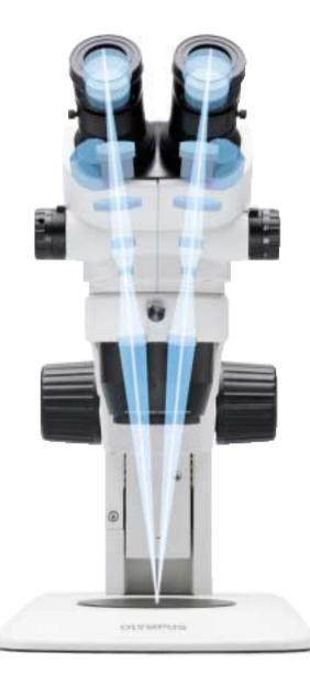
The Greenough optical system has two zoom optical paths inclined at an inward angle. This enables a more compact microscope design while maintaining high performance.
