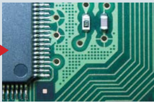
Right-quadrant illumination of PWB
