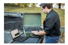
The TERRA II analyzer from Olympus Scientific Solutions is the successor to the world's first commercial battery-operated, portable XRD. This analyzer has a 6-hour battery life and a sturdy, weatherproof case for rapid in-field analysis of both major and minor mineral components.
